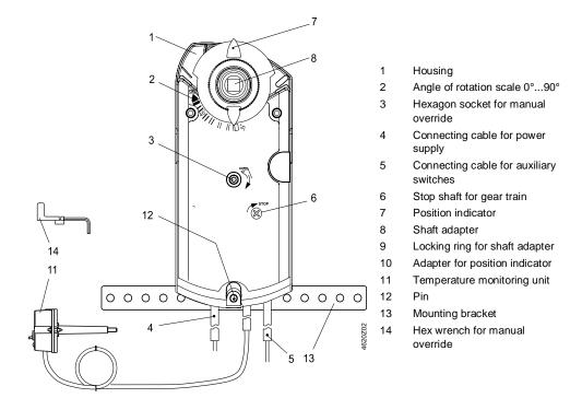
Arrangement for shaft adapters
