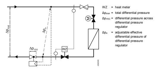
In cases where the required differential pressure value is between two spring ranges (red, yellow), it is advisable to choose the range with lower effective differential pressure  $\Delta p_w$  values to ensure the sensitivity of the differential pressure regulator.
