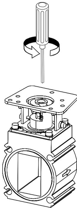
Use the Allen key to turn back the VKP to the 0° position. Turn counter-clockwise.
