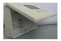
Connect the bus cable to the screw teminals.
