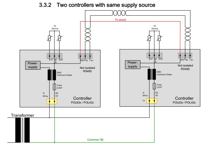
Both RS485-Interfaces can be referred using the common G0 connection. In this case, you must disconnect the REF:
