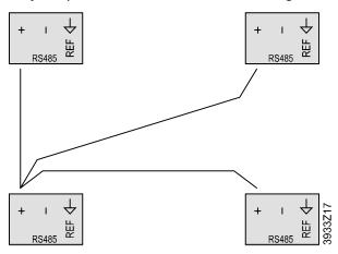
Note on figure: Only one line + (A+) is shown in this example.
