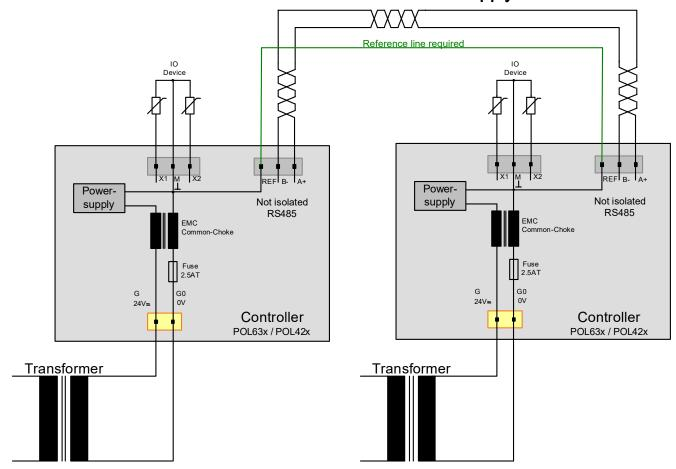
Use the REF line for proper operation of the RS485 bus if each RS485 node has a separate, isolated power supply.
