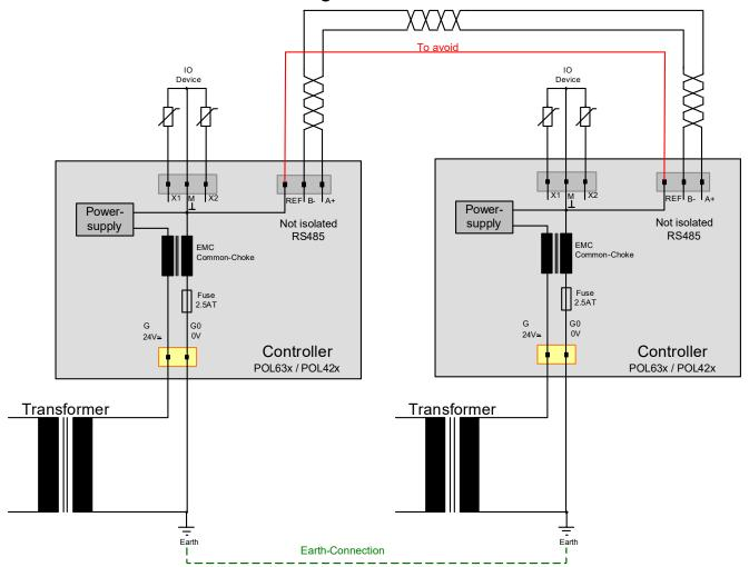
Both RS485-Interfaces can be referred using a low impedance ground connection. Disconnect the REF in this case:
