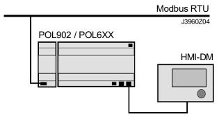
Connect Modbus module Proceed as follows to connect the Modbus module to the Modbus bus via RS485:
