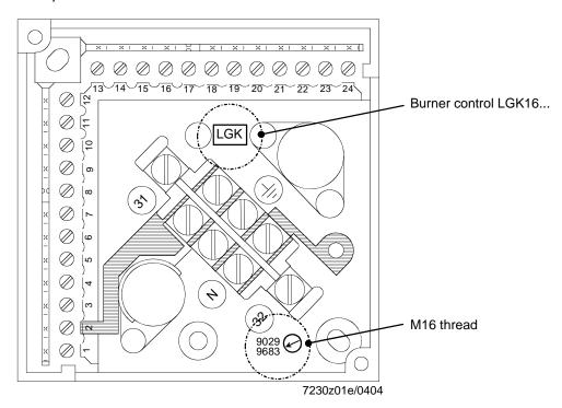
Pg11 thread: Marked 9029 on the plug-in base (refer to «Dimensions»).
