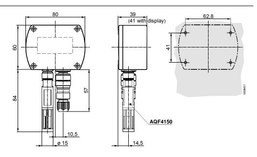
Dimensioning without (with) LCD-display Dimensions in mm
