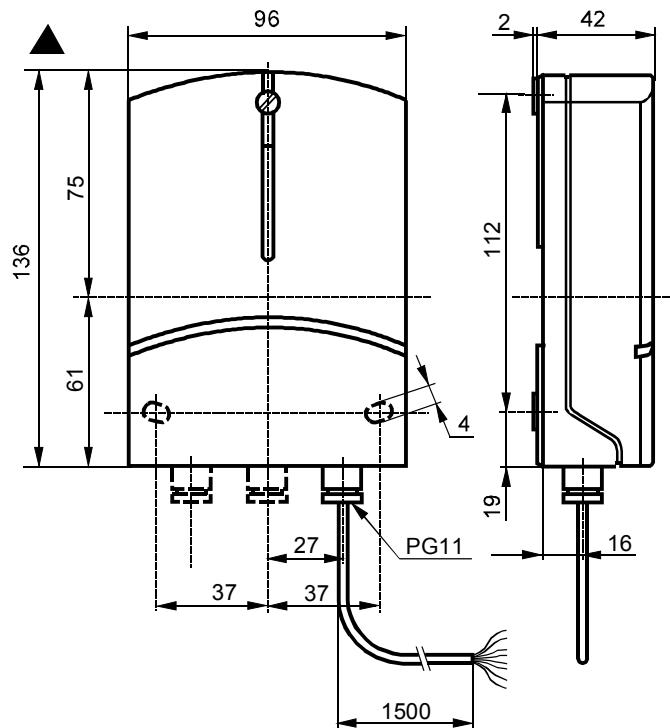
**Minimum space for fitting the address plug:**
