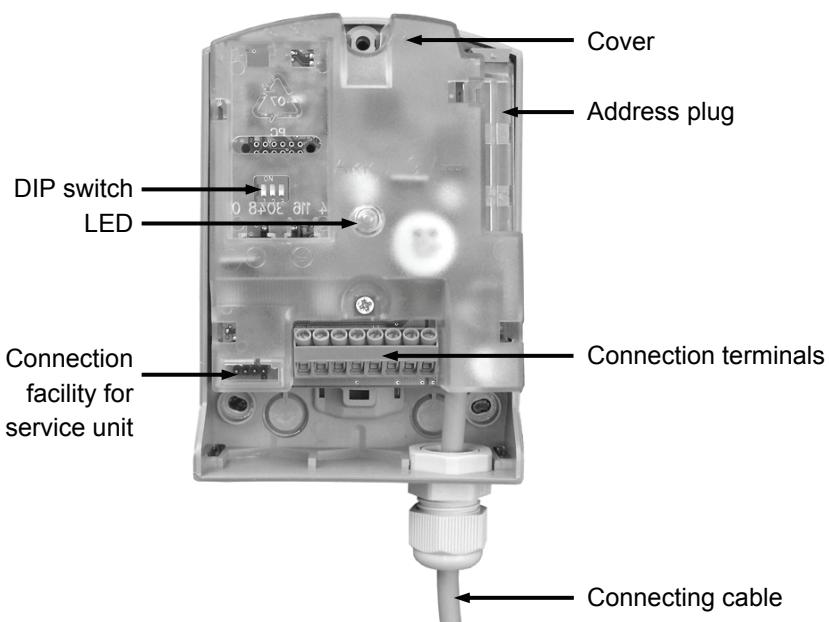
The connection diagram is printed on the inner side of the cover.
