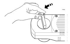
Releasing the lever manually
