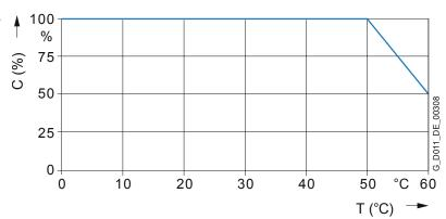
T (°C) = ambient temperature C (%) = permissible output current
