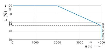
H (m) = installation altitude above sea level U (%) = permissible input voltage
