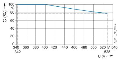
U (V) = line voltage C (%) = permissible output current
