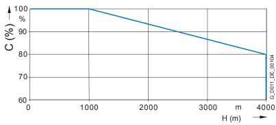
H (m) = installation altitude above sea level C (%) = permissible output current
